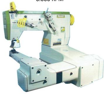
Feed off the arm heads for assembling seams on a wide range of fabrics.
